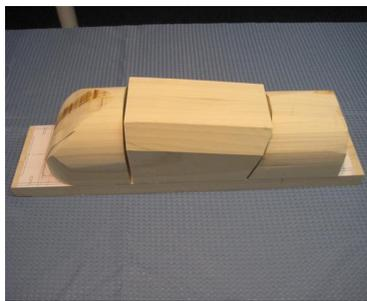
*The plywood templates are placed back in between the blocks and the surface of the blocks are now worked in by hand using a block plane and spoke shaves.*
