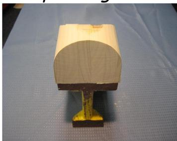
*The front block was then cut and sanded to shape in the plan view using a paper plan fastened to the bottom of the block.*
