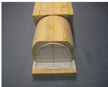
*The front 1/8" plywood template was cut and sanded to the paper print attached to it which shows the canopy shape at it's highest point in the front view. This template was positioned in place and temporarily attached to the front of the middle block.*
