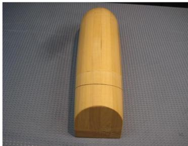
*A wood ring was constructed to surround the vac former when it is placed in the vac forming machine. This ring will aid in drawing any webs or wrinkles away from the surface of the part. The rear edge draft angle was also increased.*
