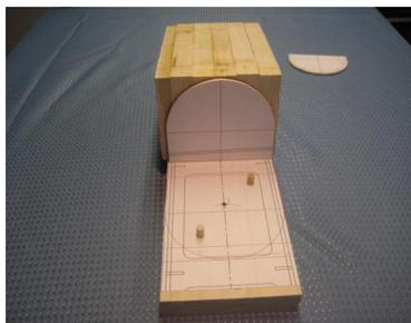
*The front poplar block was positioned on the base with the rear face of the block positioned against the plywood template that was attached to the middle block. The front block was then fastened and doweled to the base. The front block was rough cut to the high line shape of the canopy shown in the side view paper plan attached to it.*
