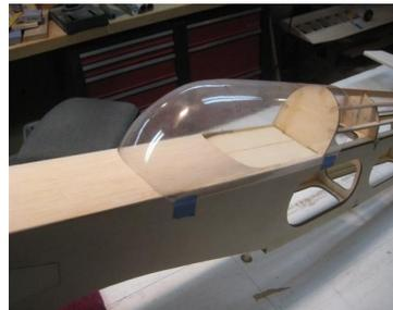
*The trim line on the prototype vac formed canopy was finalized and placed on the vac former. The final trim line was then scribed from the part onto the vac former. This scribed trim line will be transferred onto the production parts during the vac forming process.*
