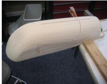
*The rear end of the rear block is cut on an 24 degree draft angle and the surface of the blocks is now finish sanded. The wood is sealed with multiple coats of shellac and sanded between coats. The approx. canopy trim line is laid out in fine line tape.*
