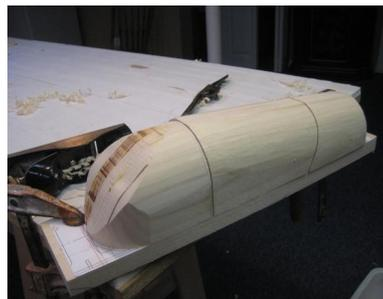
*The roughing of the surface of the blocks continue, controlled by the plywood templates and the overall shape of the base.*
