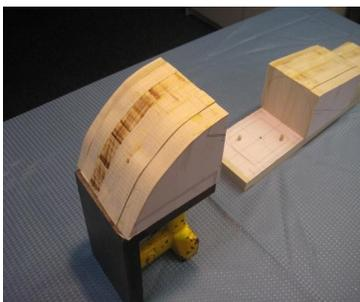
*The plywood template which shows the canopy shape at it's highest point in the front view was used to mark an outline on the front block. The front block was then cut and sanded to shape using the marked line as a guide.*
