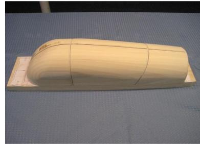
*The surfacing of the blocks are now in the finalizing stage and the front surface of the front block is extended down to the bottom of the wood base.*
