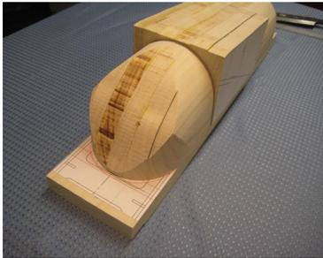
*At this point all the blocks are fastened and doweled to the wood base and the excess wood on the middle and rear blocks are removed by table saw and band saw.*
