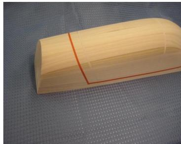
*The wood blocks are now considered a vac former ready for vac forming prototype parts.*
