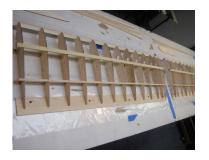
• Place the main top spar in the top notches of all the ribs, lining up the beveled end of the top spar with the beveled end of the bottom main spar using the dihedral gauge. Glue in place.
