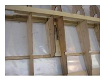
• Cut, fit and glue in place 1/4" x 1/2" spruce reinforcements for the servo mounting screws on the top of the servo trays at the forward and rear of the servos opening.
