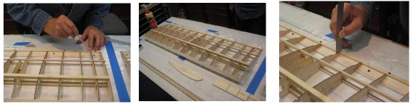
• Cross cut all webbing from 3/32"x3"x36" balsa wood sheet stock. The front webbing length is 1-3/4" long, and the rear webbing is 1" long. Nine piece each is required on each wing half to fill nine outer bays.
