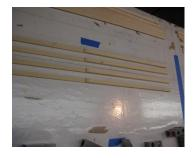
• Once the glue is dry, the sistered ends of the main spar subassemblies should be cut and sanded on a 1 degree angle as shown in the photo. Care must be used to form the <u>proper angle direction</u> on each of the sub-assembled spars. Use the dihedral gage to mark and check the angle. Set these parts aside for the wing assembly.
