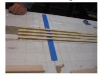
Mark and shape the rear trailing edge by beveling the <u>top surface</u> of a balsa 1/4" x 1/2" x 36" stick. See sketch & photos.
