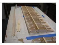
• Place and glue the preshaped balsa trailing edge (1/4"x1/2"approx. 36" long) on top of the trailing edge sheeting and at the rear end of the ribs. Make sure it is proud of the center line.
