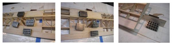
• Glue the laser cut plywood wing tips to both panels.
