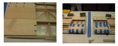
• Glue two 3/16"x3/16" top forward spars into these slots and in the notches of all the ribs.
