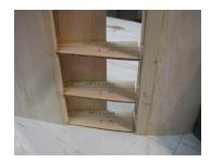
• Cut the supplied pre-made cardboard tube to 11 3/4" in length. Slide the tube through the holes in the center wing ribs up to and just through the 2<sup>nd</sup> W3 rib, and glue in place.
