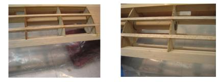
• Trim all components flush to the surface of the W1 rib at the center, and to the outboard surface of the last W5 rib.
