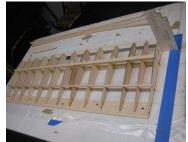
• Place and glue the balsa leading edge (1/2"x1/2"approx. 36" long) into the notches in the ribs . Make sure it is extended proud of the W1 root rib.
