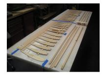
There are parts that need to be cut and assembled into sub-assemblies prior to the actual assembling of the wing.
