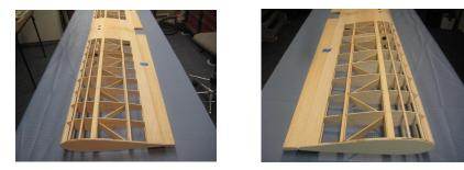
Note: Repeat the build sequence to construct the opposite wing panel if you are building the wing halves on a smaller work surface. <u>Be careful not to</u> <u>build two like panels</u>.
