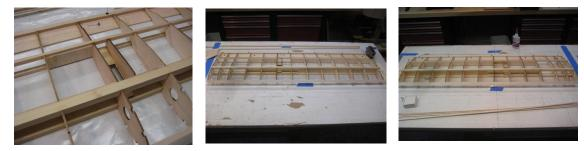
• Cut, fit and glue in place the diagonal wing braces, made from stock balsa 3/32x3/4x 36", between the webbing of the front and rear spars, centered to leave clearance at top and bottom.
