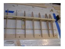
Place the W4 (partial) rib "bottom" down flat on the work table between the main spar and the forward edge of the rear 1/4x1/4 spar, against the aileron servo tray (trapping the servo tray). There should be a 3/32" gap between the front edge of the rib and the main spar. Glue in place.
