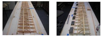
• Cut, fit and glue the rear top sheeting between the center line and the outboard side of the W2 rib.
