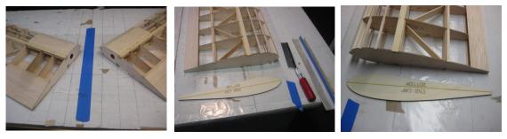
• Join the two (right an Left) wing panels together using the plywood laser cut dihedral brace installed between the main spars. Care must be used to ensure there is no interference between the wing panels and the dihedral brace providing a snug fit. When satisfied with the fit between the two wing panels the following steps should be taken.
