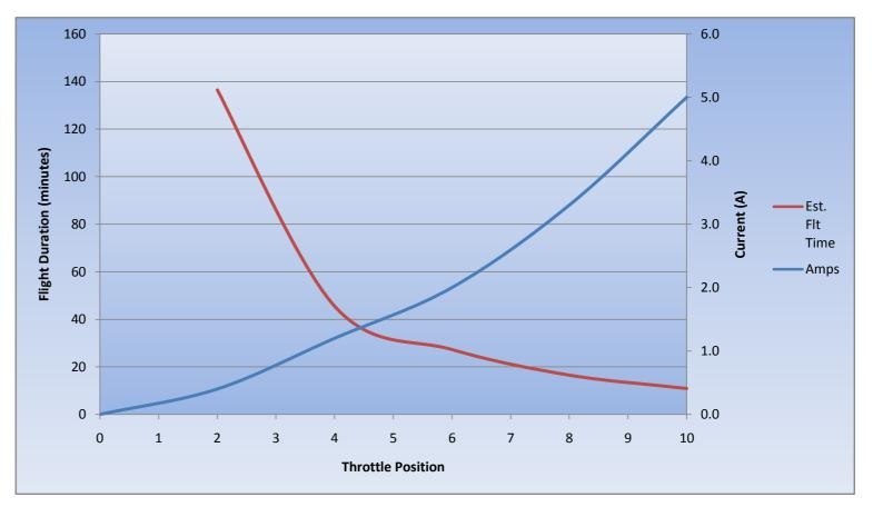
As measured on test stand at RCCD Ground School - April 2009
