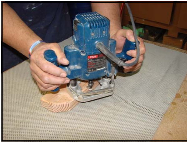
Edge routing with a bevel cutter
