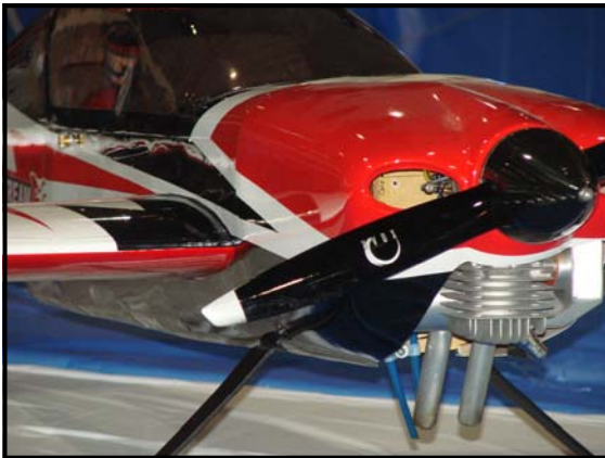
Business end of Lou Tisch's Schach 342 DLE 55 cc gas engine
