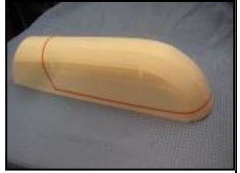
Canopy pattern for vac forming
