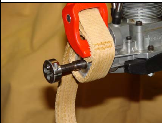
Strap Wrench in place to hold prop shaft for cutting threads.
