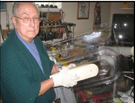
Norm forming & pulling a canopy.
