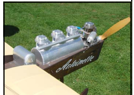
Jim McCoul-Scratch built Antoinette-96" Wingspan-0S.91FS for power with dummy engines heads.
