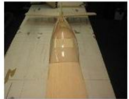
Canopy pattern for vac forming
