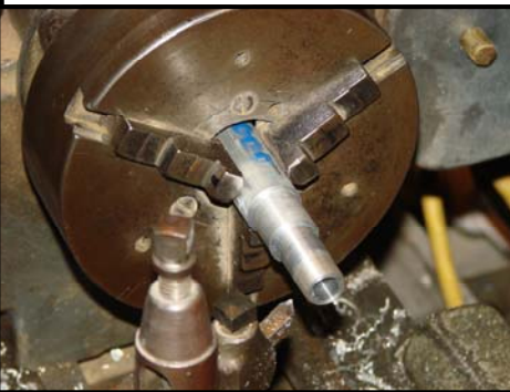
Aluminum rough cut to diameter.
