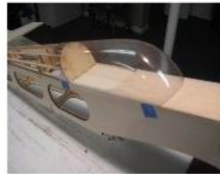
Installation step for the canopy.
