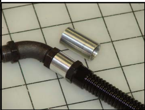
Sleeve parted off, chamfered .
