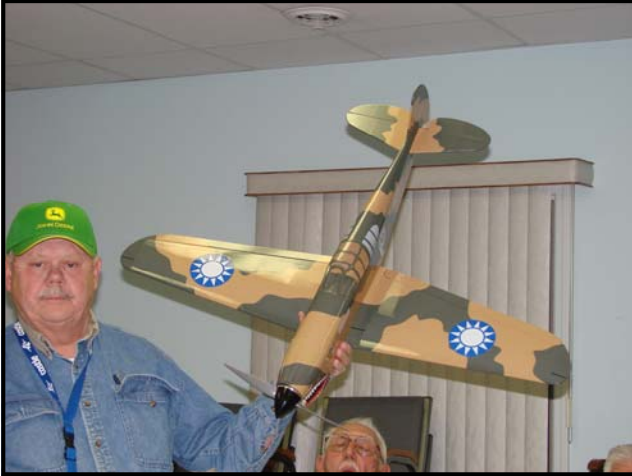
Ken Sulkowski-GP P-40 Warhawk 39" wingspan-Elec. 500 watts, 11.1 volts
