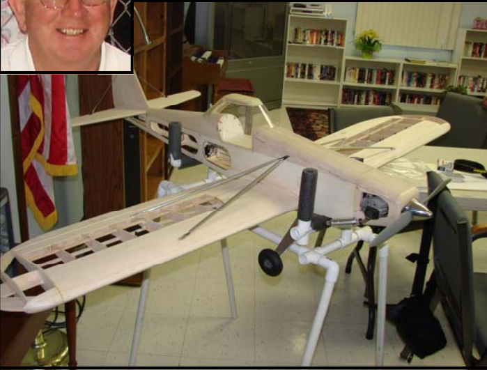
Noel Hunt-Starduster (scratch built) 70" ws, OS.91FS, Flaps & Tow Capable
