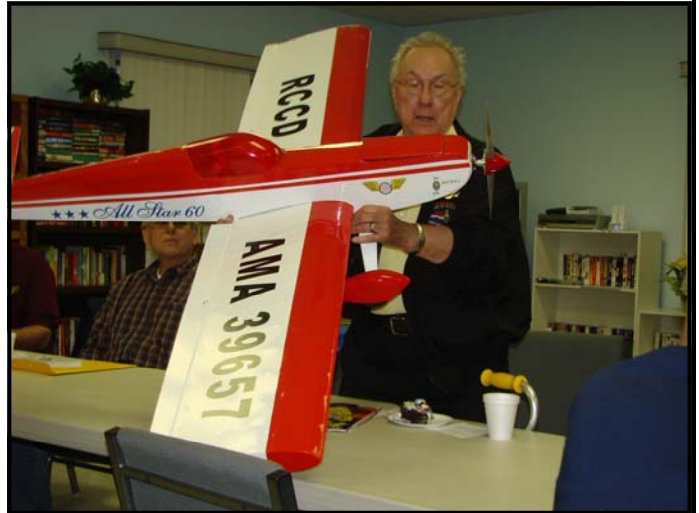
Norbert Zielinski-All Star 60 (scratch built) EP-500 ma Battery— 62" wingspan
