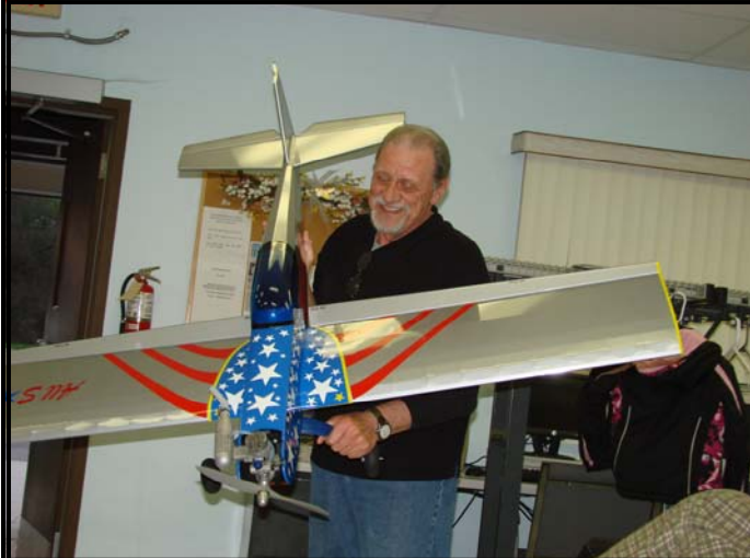
Pete Mlinarcik-All Star 60 Project Prototype 70.5" wingspan—OS.60SF for power
