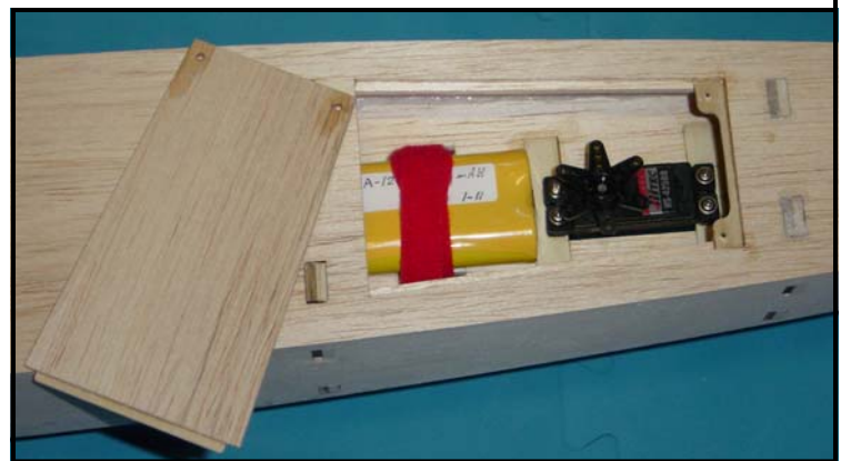
Battery hatch in the fuselage behind the wing area. In this case the elevator servo occupies the same hatch.
