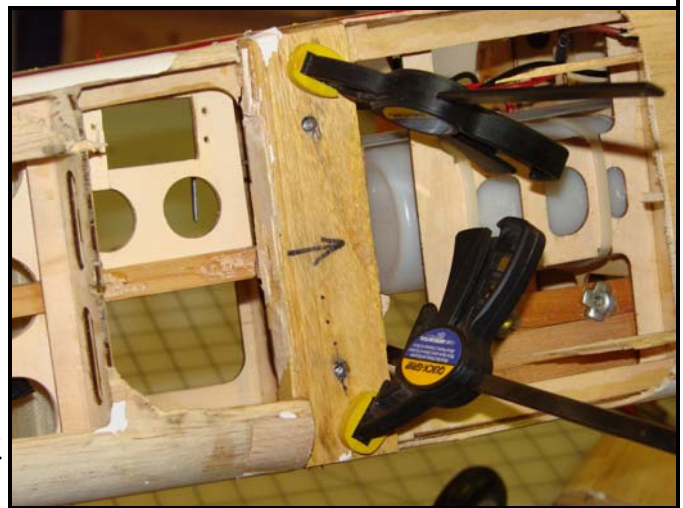
LG mounting plate clamped and epoxied in place.
