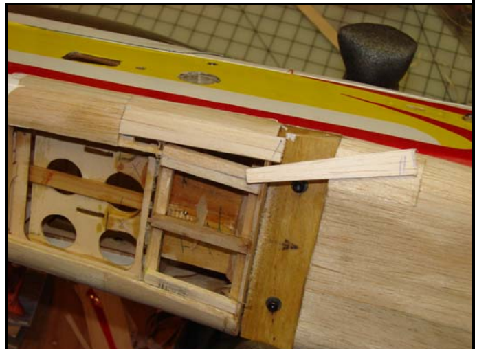
Planking begun on undercarriage contoured section.
