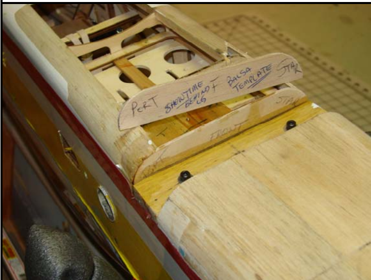
Front lower cover set into place & contour template installed to allow for planking behind the LG plate.
