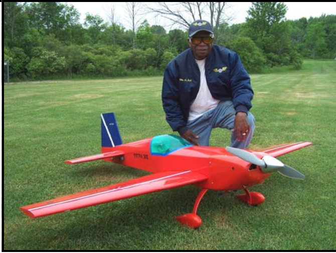
Willy McMath, one of our club founders, flying his scratch built Extra 300XS. It weighs about 17# and flies well with a Turnigy Electric Motor.
