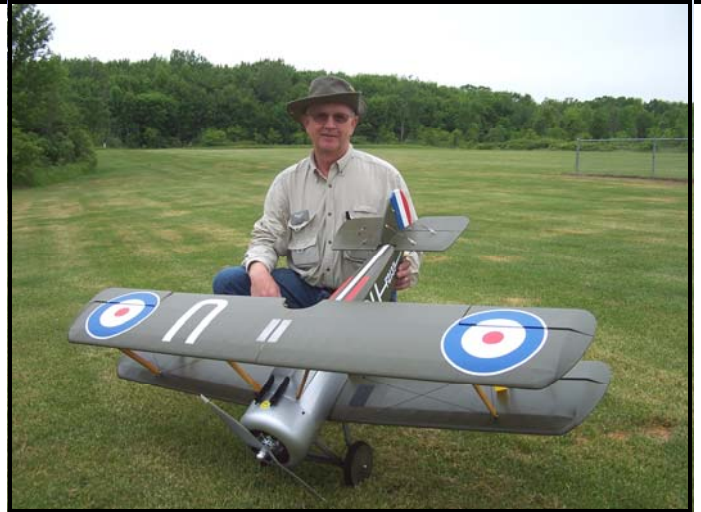
RCCD Club Vice President, Noel Hunt (New IMAA member), with his 7#, 61" wingspan, Hanger 9 Sopwith Camel with a Rimfire 55 motor and A-123 Batteries. Noel says that this is the most challenging model he's ever had to land with about 60% of landings being "scale landings"...tipped on the nose. As I understand, that's one reason cockpits were padded.
