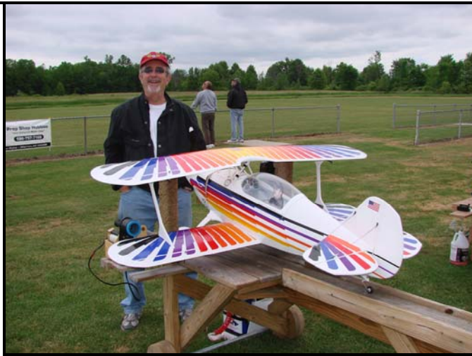
Herb Mills with his 27.5% SkyShark Christen Eagle, outfitted with 8 servos, Futaba 2.4 gig radio and a Moki 2.11 2-C engine with Sonic Tronics on-board-glow. This is a very well behaved model and Herb has just gotten it dialed in.
