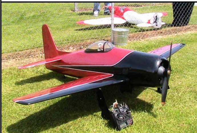
Keith Shaw’s 81” Bearcat uses 10s2p A123s, an Astro 60 brushless motor and a 3:1 belt drive. The 1/5.5 scale model weighs 14lb
