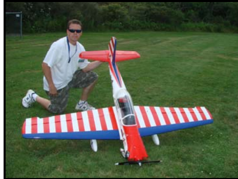
Dave Durocher-GP Super Chipmunk 81' WS-OS200FS-18x8 MAS Prop
