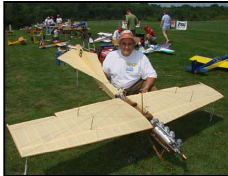
Jim McCoul— scratch built Antoinette. It's powered by an OS.91FS. 96" WS & take special notice of the carved cylinders to match the motor.
