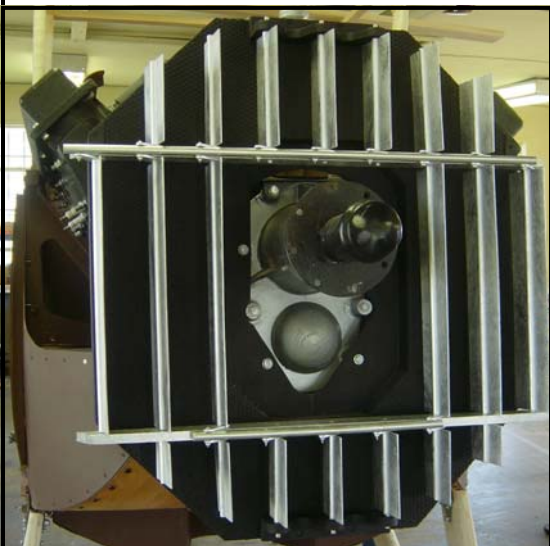
Adjustable shutters to provide temperature control for the engine. (pictures to L & R)
