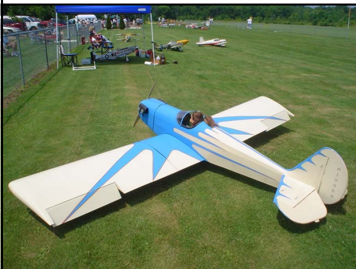
Vince Blasky Plane: 1/2 Scale Space Walker, 40#, WS-165" Light Ply & Balsa Construction Engine: Quadra 100 Radio: All Futaba (T6XA) Finish: Stitts & C-21 Covering and Dope
