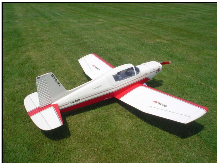
Chris Tucker Plane: Morrissey Bravo by Sig, WS-84", Length-76" Engine: US Engines 41, Zinger 18x8 This is Chris's third airplane, & he's had it for 5 years and logged 100's of flights on it. It's covered in Super Coverite and painted. It has strobe lights and the pilot is coupled to turn with the rudder.
