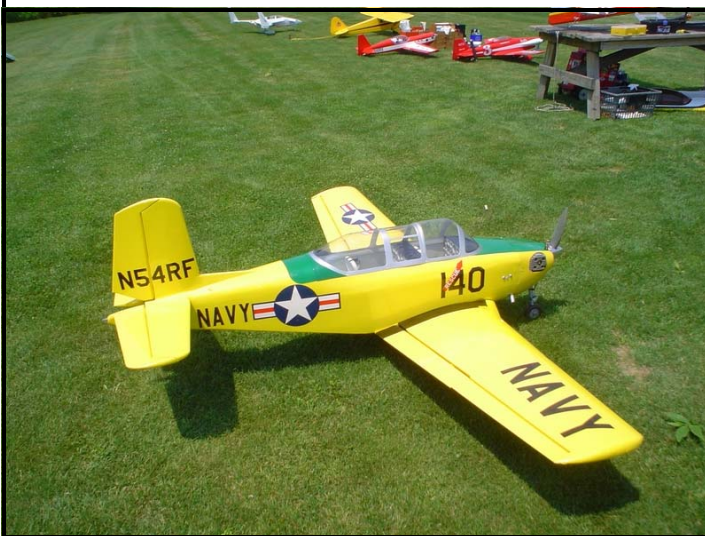
Ken Thompson Plane: Top Flight T-34 Built by Bill Hackett WS-80", Scale Cockpit Kit w/ Instruments Engine: Super Tigre 2300 Radio Equip: Hitec Digital Servos (120 in/oz torque) & Hitec Receiver Battery Pack: 1650 mAh 5 cell Receiver Pack
