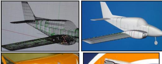
....A quick look at the work Dave did with the CAD program. After tweaking the wire frame to match the full scale plane, it was surfaced to give an idea of how the completed plane would look and allow for proofing of the contours.
