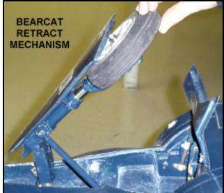
In the gear sequencing set up, Dave designed another rod and stop (see left picture by finger) that would hold the tire clamped in position when closed. With the solution in place, the plane was ready for competition and the air.
