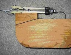
the forward momentum releasing the spring clip to close the switch contacts to the alarm device
