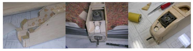
Here are a few sequence pics of the progress on my 3rd Legacy. I've also moved the wing position to better balance the model without having to add non-productive weight. This has necessitated a bit of reconfiguration & design but it will pay off in the end.
