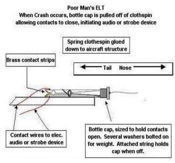
This is a picture of my test model. As you can see. I used small bolts and nuts as the contacts. The small bottle cap with weights attached hold the contacts apart until the forward motion of the aircraft is suddenly stopped, whereas the weighted bottle cap continues
