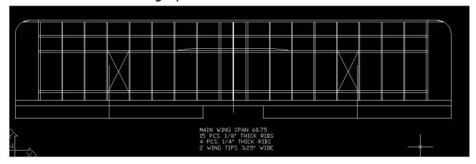
This option has a 67" wing span and is like the option above but with an additional 1/8" thick rib added to each side of the wing. It has a total of seventeen 1/8" thick ribs and four 1/4" ribs, with 3.25" wide wing tips. Note, the ailerons travel outboard with the edge of the wing and the space between the fuselage the inboard edge of the aileron just increases.
