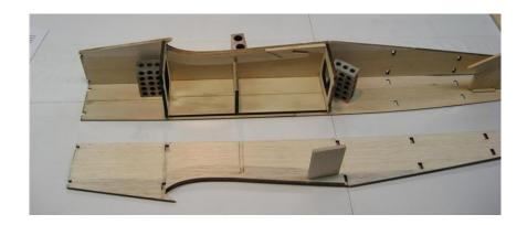
\*Dry fit and position both fuselage sides using the side tabs of Formers F2 and F4, and allowing former F3 to fit into the vertical slots of the reinforcement saddle. The 1/4" plywood wing attachment cross member will also have to be fitting in between both the fuselage sides in front of former F4 and into the reinforcement saddle. Keep in mind, I did mention frustration and dirty words.
