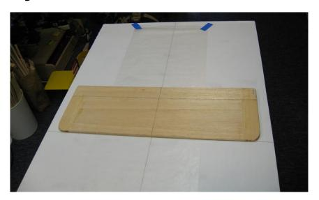
\*The bottom fuselage panel assembly is made by gluing the rear edge of the 3/32" plywood front bottom fuselage panel to the front edge of the 3/32" balsa rear bottom fuselage panel, making sure the side edges line up.
