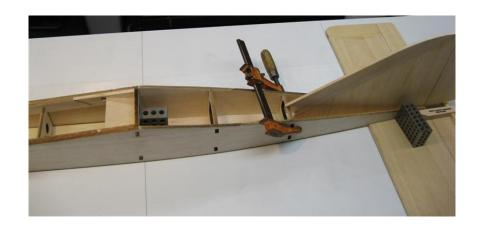
\*Make sure the tabs in formers F 5 and F6 are in the slots in the fuselage sides and the fuselage bottom. The rear inside edge of the fuselage sides should be dubbed or chamfered to match the vertical fin to provide a larger glue surface.
