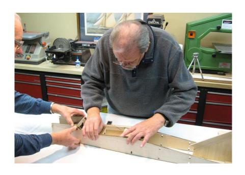
\*This is the starting point of the assembly of the whole fuselage. When you are fully acquainted with this assembly sequence, then disassemble the dry fit and start the gluing process. Glue in only the parts mentioned above. Make sure you don't glue the fuselage sides to the fuselage bottom rearward of F4 and in front of F2. Keep your gluing confined between F2 and F4.
